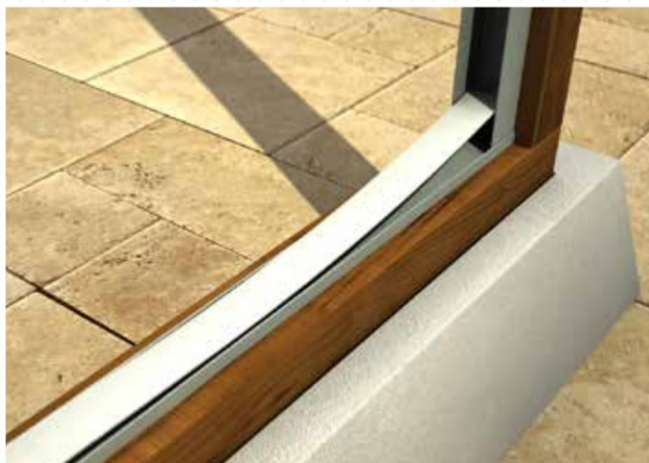
**5.** The first glass element must be centered on the point previously marked. You will introduce it into the upper profile first and then into the bottom one.
