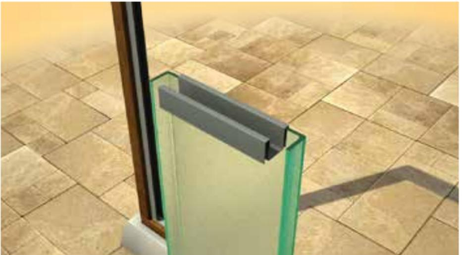
**6.** Place U - GLAS starting from the middle and continue to the both sides. Start first with the back glass element, fix it into the upper profile and then into the AC support below, that was previously placed in the middle. Add the other glass plates strating from the middle toward the sides.
