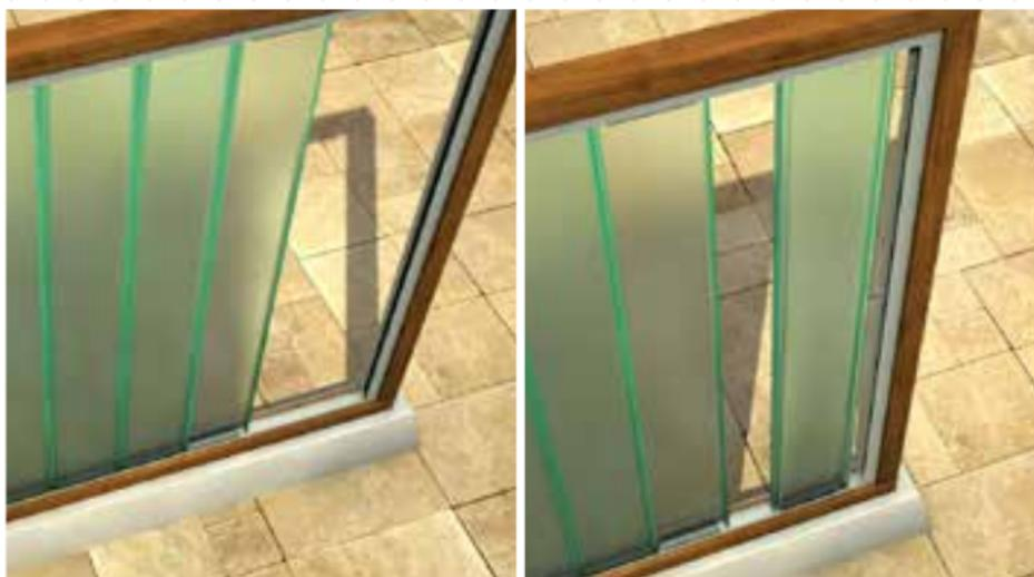
**11.** At the end, for the elements jointing, fill in the spaces between the glass elements and the spaces around the aluminum frame with silicone.
