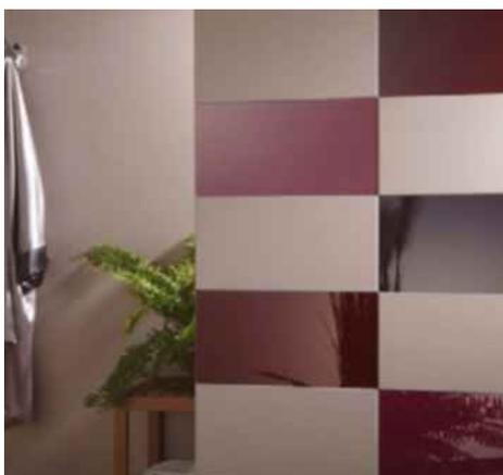
When products are mounted as a banner, keep a minimum 3mm margin between the two structures. To preserve the original stylish appearance of each product, the glass should not be fitted with the enamelled side (side 1) facing outwards. A Heat Soak heat-treatment Test compliant with standard EN 14179 is always recommended for façades and edge-to-edge or flush fitting.
